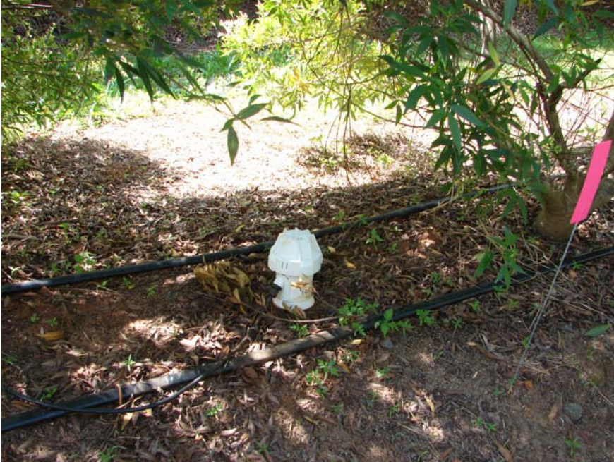
Photo 2: Location of the Enviroscan probe between the irrigation drip lines
