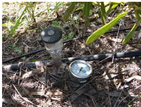
Tensiometer installed in a Protea crop
